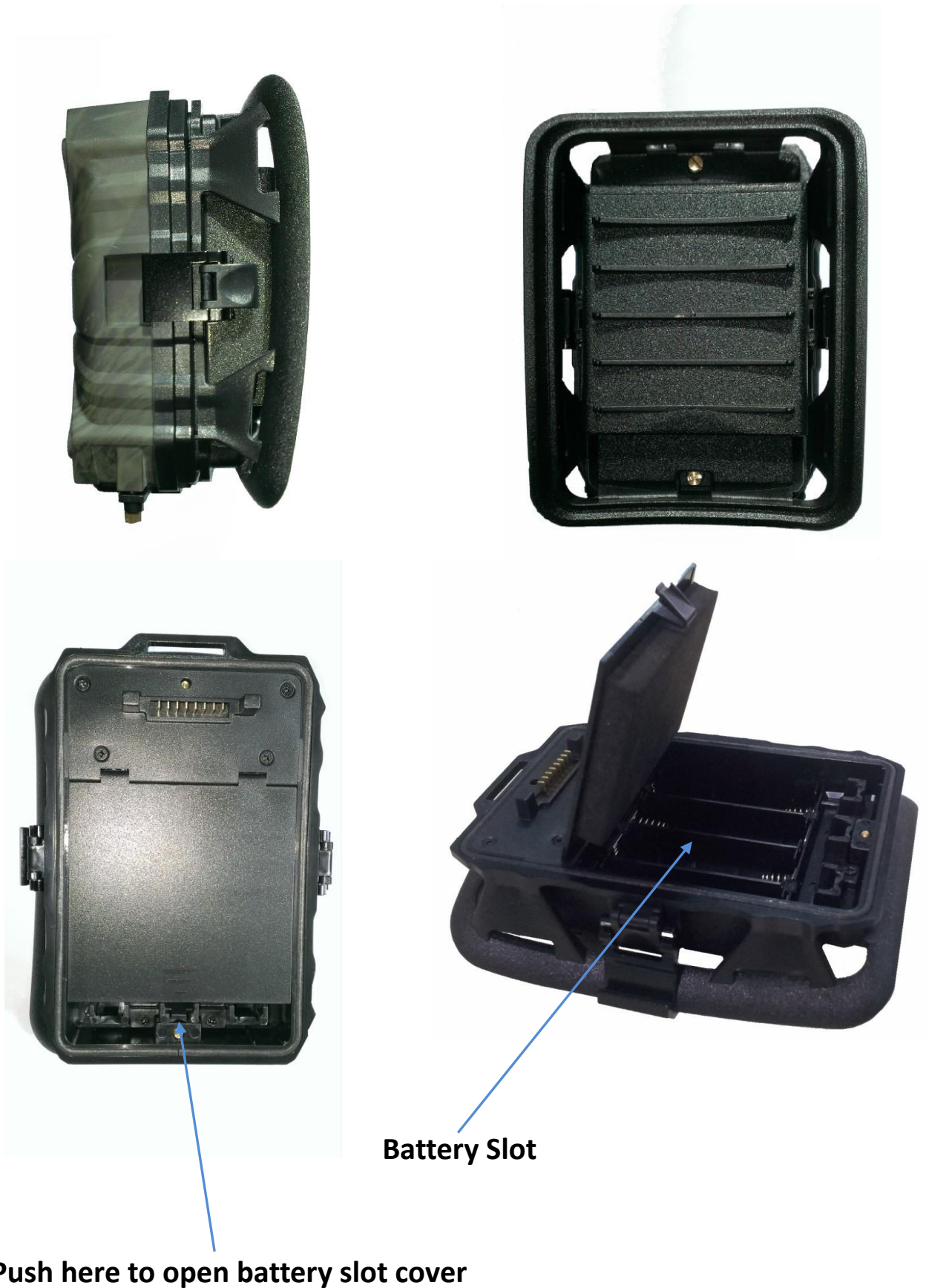
2.3 Figure 3.3: Side and Back View of Camera
